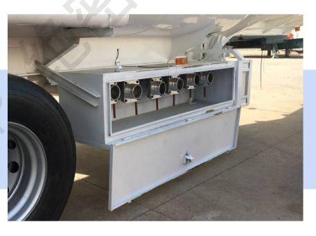
Normal discharge valve has only unloading function. When loading, it needs to use manhole on top. It is dangerous for workers in some extent.
