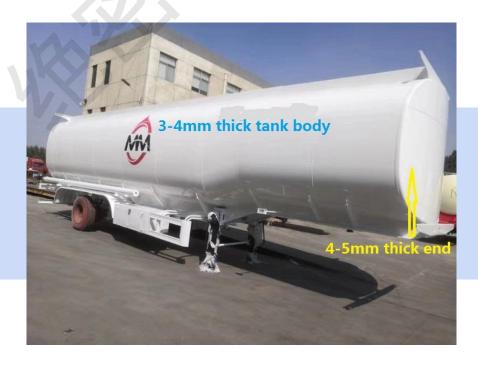
Tank thickness is 4mm, and end plate is 5mm, to save cost, but durability is not sure when use.
